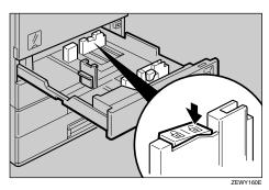
**5** While pressing the release lever, adjust the side guides.
